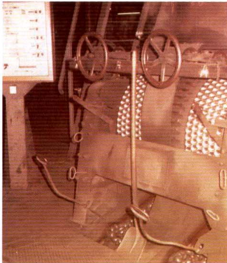
Photograph 11.15 — Industrial briquetting press. Note bitumen-bound briquettes at the base of equipment
