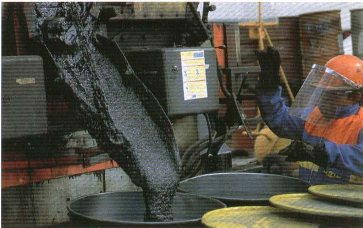
Photograph 11.2 — Encapsulated spent catalyst being packed into metal drums
