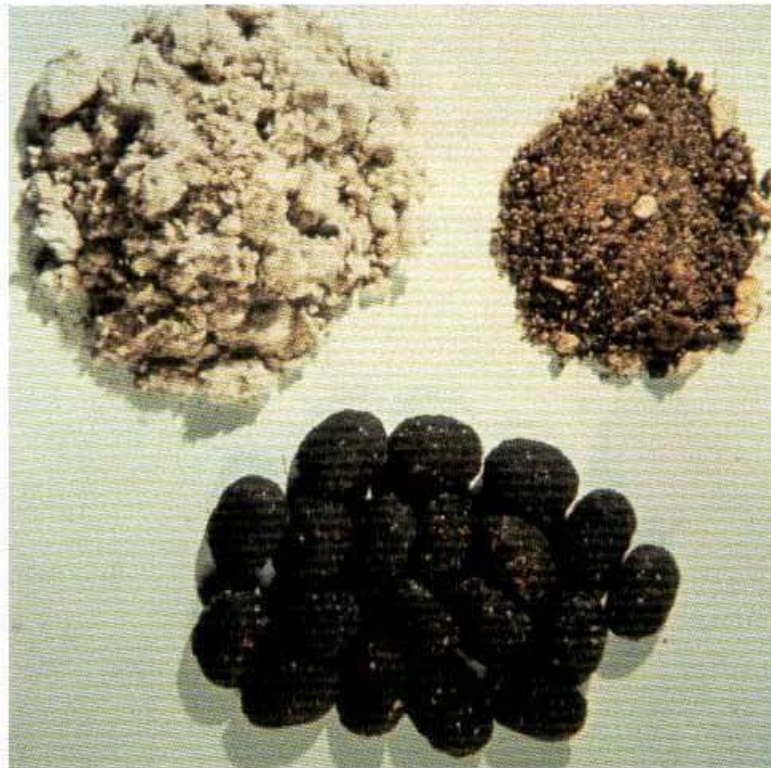
Photograph 11.14 — Recovery of industrial waste by briquetting allows materials to be easily handled and re-used in a process
