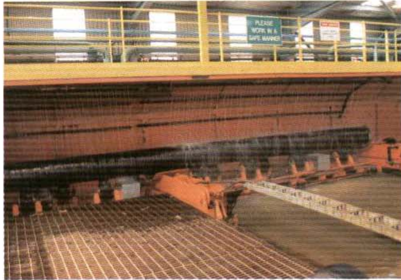
Photograph 10.5 — Coated pipes cooled by water spray prior to inspection (Photograph courtesy of British Pipe Coaters)
