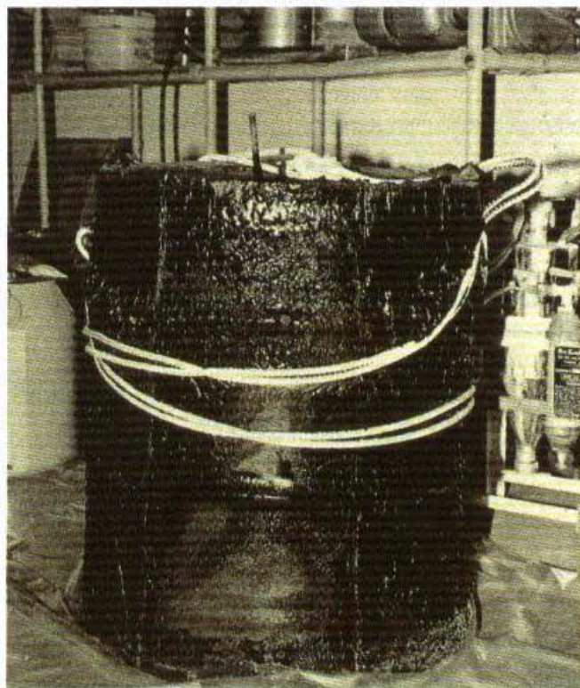
Photograph 11.3 — Drum of agglomerated radioactive waste used for leaching studies (note completely corroded drum)
